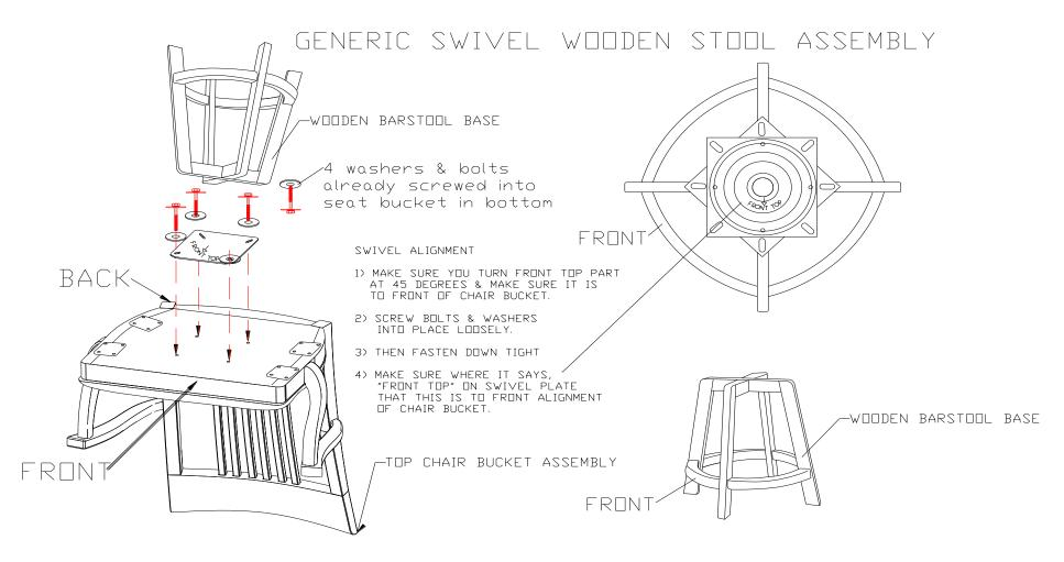
PRE-CAUTION: EVERY 6 MONTHS- RETIGHTEN THE 4 BOLTS IN THE MOUNTING PLATE. USAGE CAN MAKE SCREWS WORK LOOSE OVER TIME.
